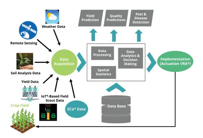
**Figure 1**: Presentation of a precision agriculture system adapted from Bhat, S. A. & Huang, N.-F. [15]. \*Acronyms: Internet of Things (IoT), Soil Apparent Electrical Conductivity (ECa), and Variable rate application (VRA).
